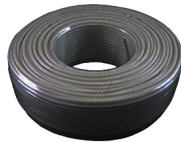
SCL-100FT-SJTW18/6-BK WHITE 100 FT. CORD, SJTW 18 AWG 6-CONDUCT ( WH/BK/GN/PU/GY + RED FOR EMERGENCY)
